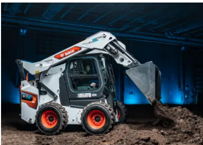
Skid Steer Loader (Bobcat)
